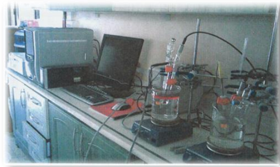
Fig. 1. Potentiostat apparatus for polarization test.
