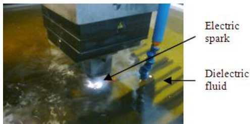
Fig. 1. Electric spark and dielectric fluid in EDM process.
