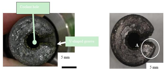
(a) Drilled hole length of 35 mm (b) Drilled hole length of 50 mm (ii) Tool wear of the drill tip
