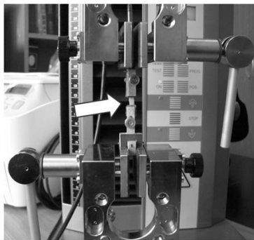
Fig. 1. The setup for uni-axial tensile tests with a universal testing machine Zwick/Roell BDO-FB0.5TS (Zwick GmbH & Co, Ulm, Germany) equipped with test Xpert software. Analyzed material sample marked with an arrow.
